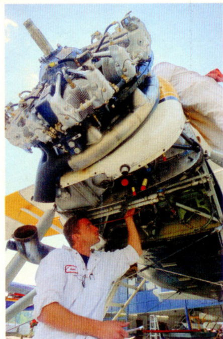
Passengers wait to board one of Kenmore Air's DHC-3 Turbine Otters at Friday Harbor on San Juan Island (above). The dock is one of several "boarding gates" where regularly scheduled service is available in the San Juan Islands. Installing a freshly overhauled Pratt & Whitney Wasp Jr. on a de Havilland Beaver (right).
